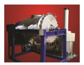
Vacuum Paddle Dryer to operate at 70 to 80° C. Innovative acquired Paddle Dryer from Dynatech Engg. Co., to dry their end product of paste type at a temperature of 70 to 80° and under vacuum. The product containing around 50% moisture is dried to powder form. The dryer is of 1000 Ltrs. total volume made of SS 316 with M.S Hot water jacket.
